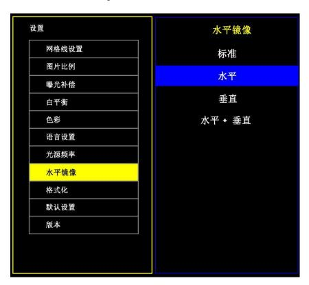
1. Press MENU to open the main menu, press DOWN to move to the horizontal mirroring option, then press OK to confirm to enter the menu; this menu allows you to select the orientation of the video image to ensure that you see the most appropriate
